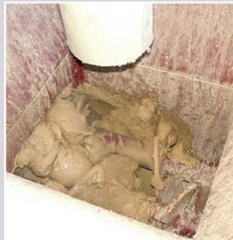
*Jarosite sludge entering the double-shaft screw conveyor*
