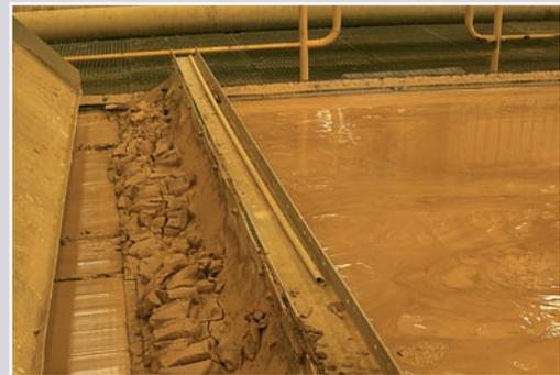
*Belt filter press with dewatered Jarosite sludge*
