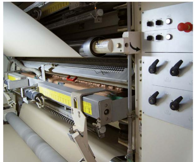
Laminating unit of a flute lamination machine (source: VDW)
