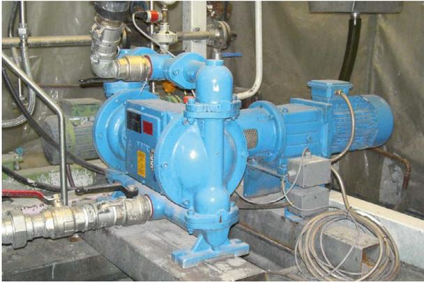
Electromechanical diaphragm pump, Type EM-040Z0300-SG for glue circulation
